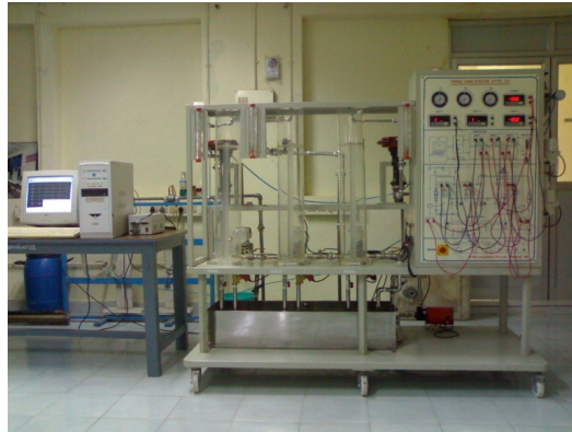
Fig. 1. Hardware Set-up of Three Interacting Tank Level Process
