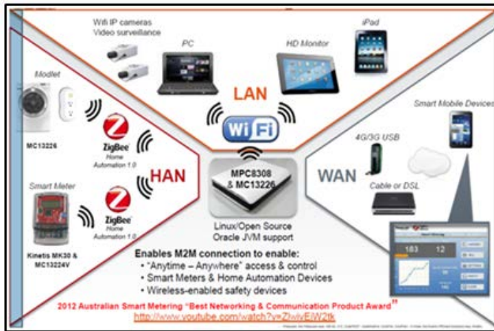
Fig. 5. Home Energy Gateway on Freescale MPC 8308
