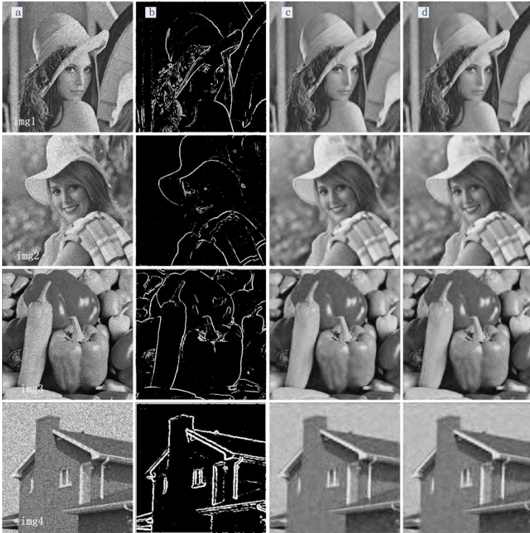
Fig. 5. The denoising results of proposed method. Row 1 to 4 is the Img2 to 4, respectively. Column (a) are the noisy images. Column (b) are the detected edges by using the IRKT. Column (c) and (d) are the denoising results of CTSofTDE and CTBDE.
