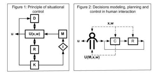
The systems R and C (Figure 2) are using the Principle of situational control and are, respectively, control systems for *modeling* and *planning* decisions.
