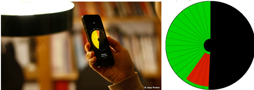
Fig. 2. The Ampul prototype [12] (left), extension of the Ampul concept (right) where solar panel production of the ‘Concept House’ is shown in green and total electricity consumption is shown in red
