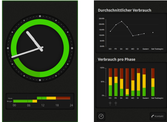
Fig. 1. Forecast view: Clock, timeline “today” and timeline “tomorrow” (left), and the feedback view: Average consumption, consumption per phase, and reward icons (right)
