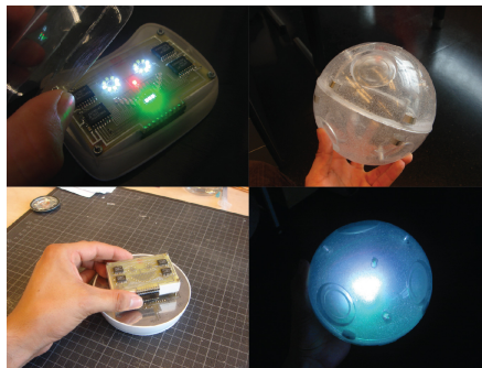
Fig. 3. KITA's main components: a) Left. KITA's face expressions and nest b) Right: rubber ball containing KITA's nest and providing sound and light feedback
