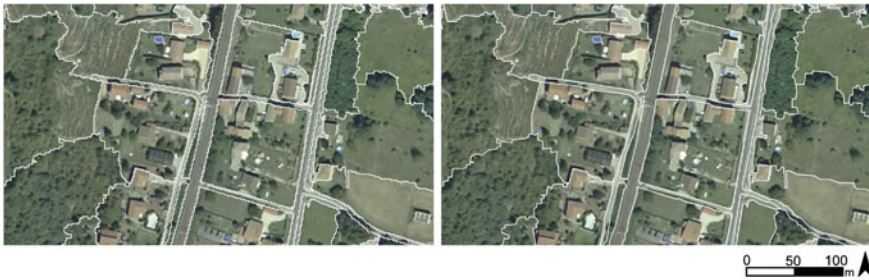
Fig. 6 Geometric simplification of image-objects
