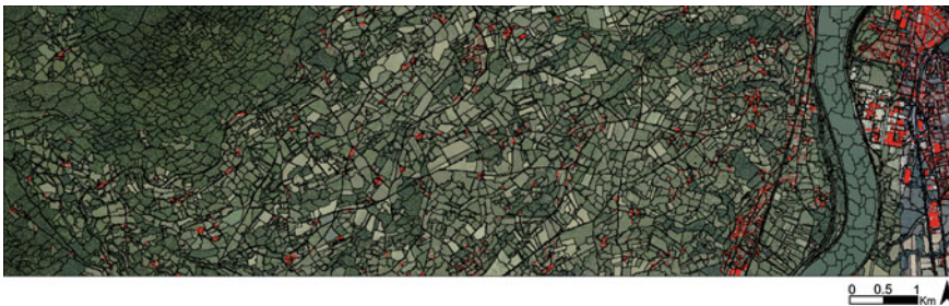
Fig. 7 Meeting between image segmentation and buildings information ( in red ) from BDTPO ® IGN
