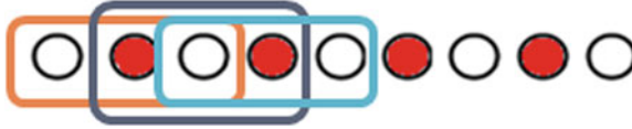
Fig. 3 Example of movement window: the data associated with each window is shared between consecutive windows. In a new window, the oldest trackpoint is lost and the most recent one is added. In this way, the mean of the coordinates evolves smoothly and is less prone to errors of data capture
