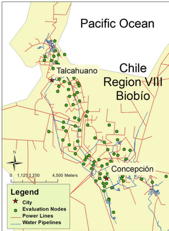
Fig. 15.1 Map of the evaluation nodes from the Talcahuano and Concepción region during the 2010 Chilean Earthquake along with streamlined transmission level power and water networks can also be averaged to find overall interdependencies and their lengths of influence
