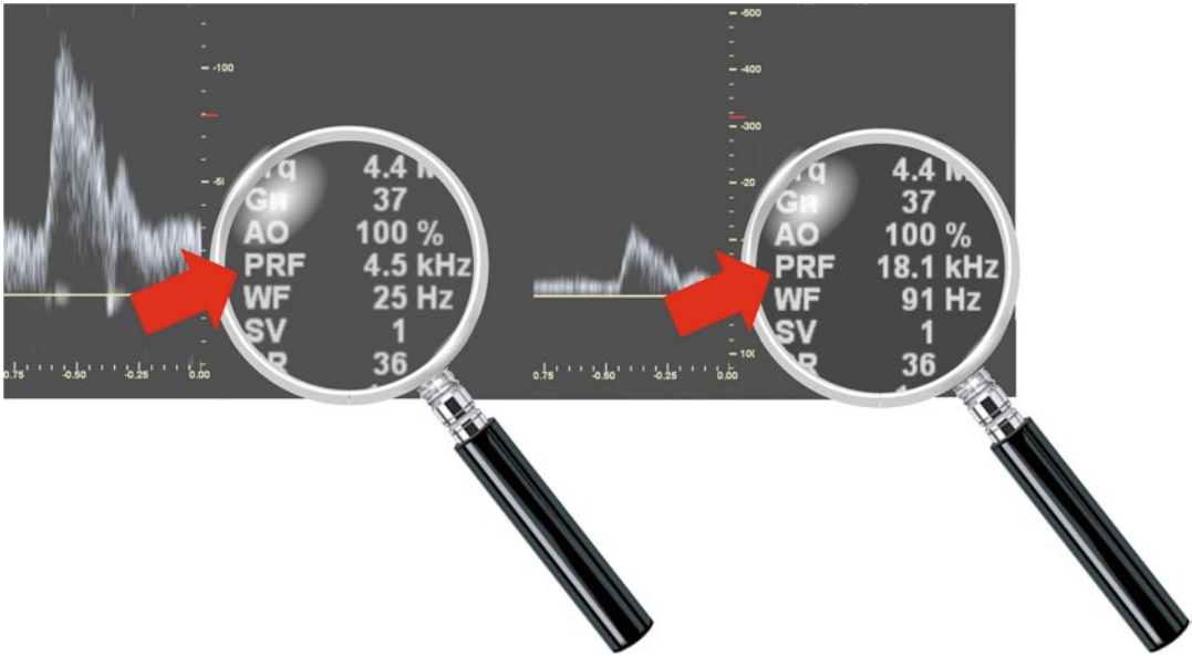
Fig. 1.18 Relation between PRF and velocity range
