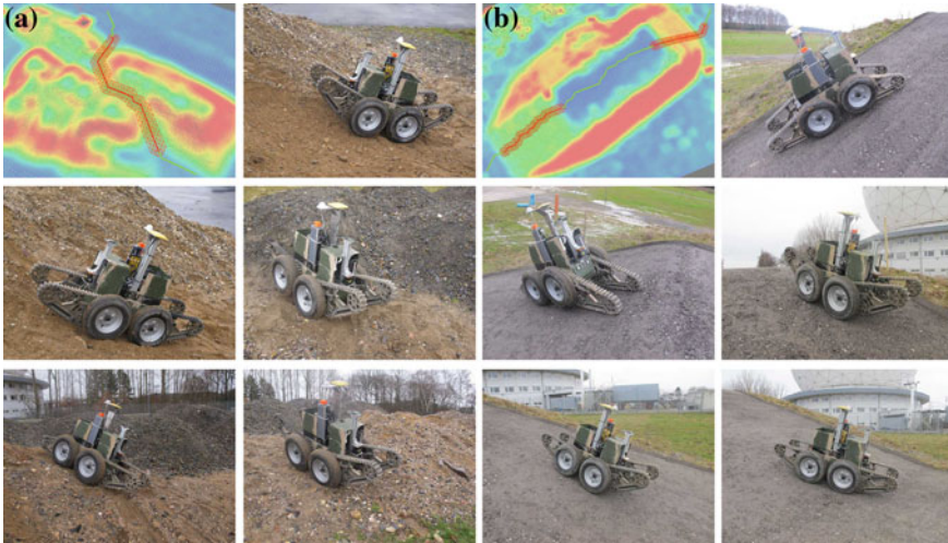
Fig. 10.9 Results of the real-world experiments. The first images depict the plan given to the robot. The other images show the robot during the execution. If the robot safety permits, configurations are sometimes applied in advanced or while in motion to avoid stop-and-go movement. a First Scenario: Hill of Rubble. b Second Scenario: “Testing Hill”
