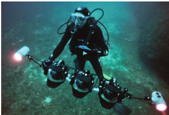
Fig. 14.7 The photogrammetric survey using three digital camera synchronized (photo Pierre Drap, all rights reserved)
