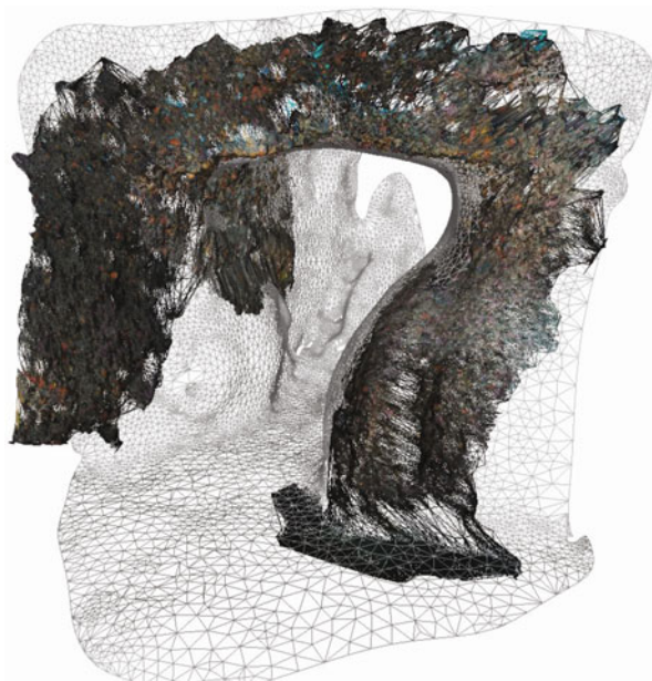
Fig. 14.8 Merging optical and acoustic underwater data
