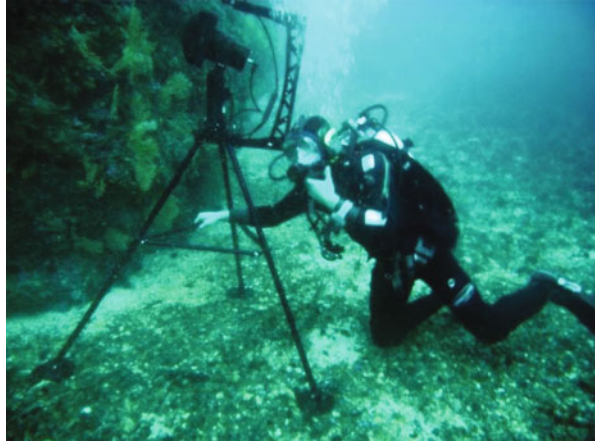
Fig. 14.5 The acoustic camera in situ, just in front of the cave—see next image—(photo Bertrand Chemisky, all rights reserved)
