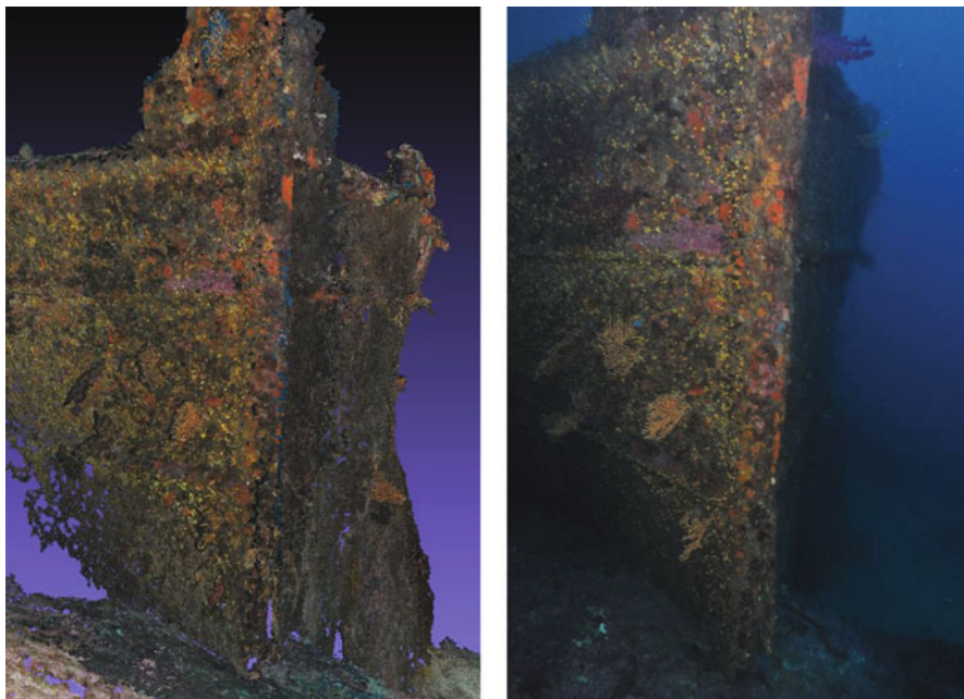
Fig. 14.10 On the right, one of the 1,221 digital photographs taken (photo Olivier Bianchimani, All right reserved), on the left, The “Liban” wreck.: Cloud of 3D points measured by photogrammetry using Furukawa method
