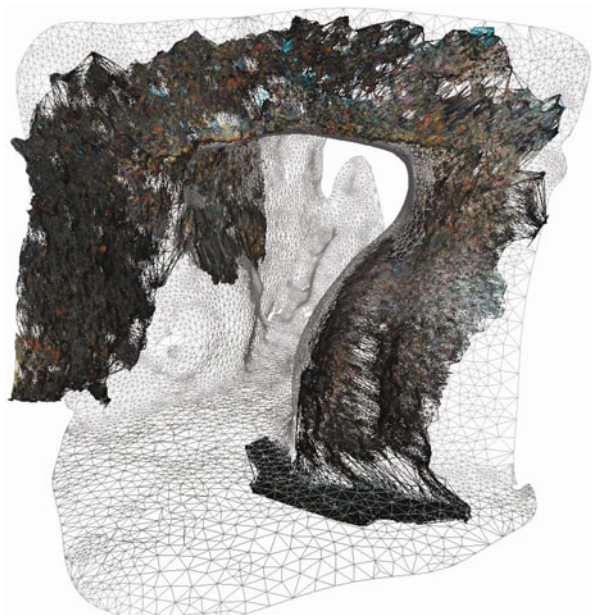
Fig. 14.8 Merging optical and acoustic underwater data
