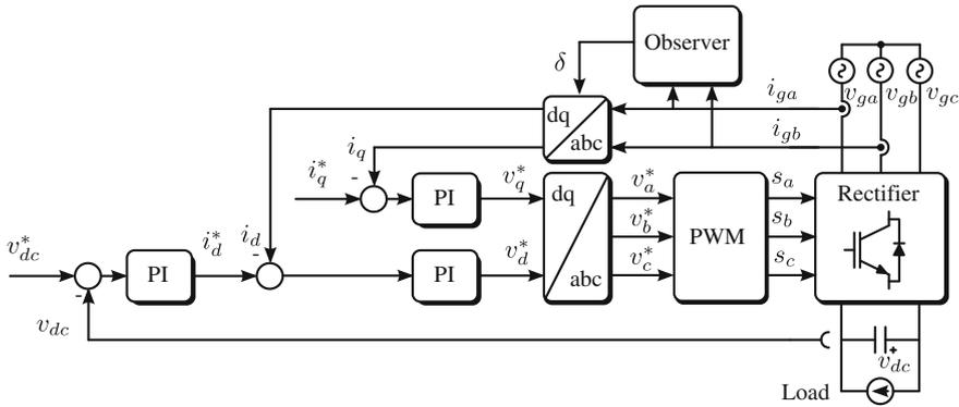
**Fig. 7** Classical control of rectifiers: voltage oriented control
