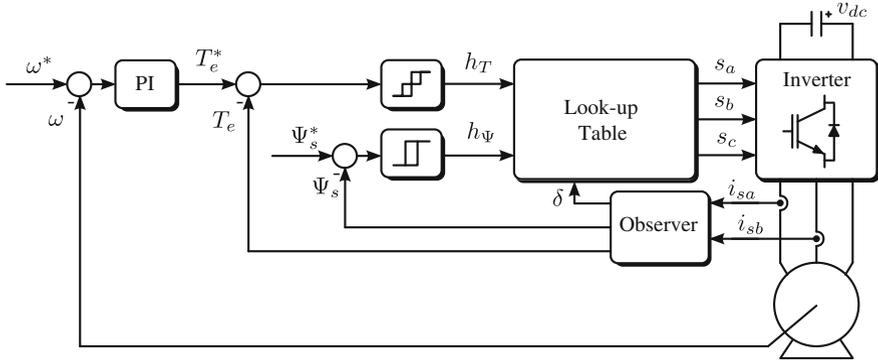
Fig. 6 Classical control of inverters: direct torque control
