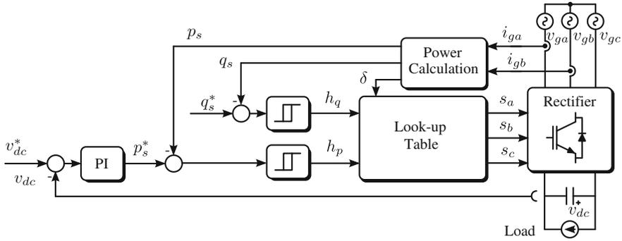
**Fig. 8** Classical control of rectifiers: direct power control
