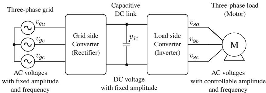
**Fig. 1** Basic structure of an AC-DC-AC power converter
