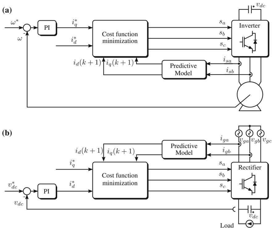
Fig. 9 Model predictive control a Inverter, b Rectifier
