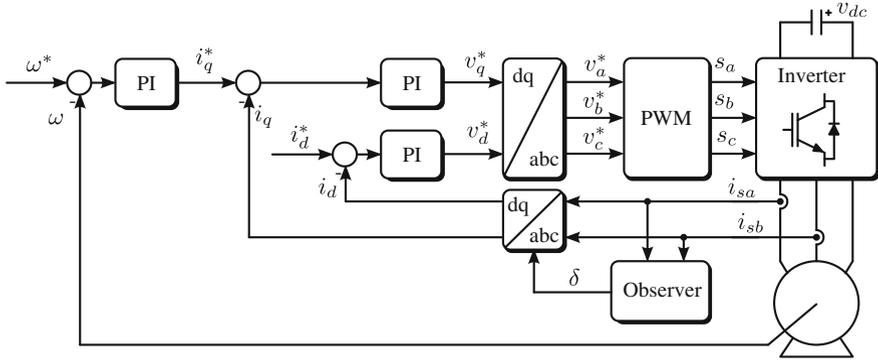
Fig. 5 Classical control of inverters: field oriented control
