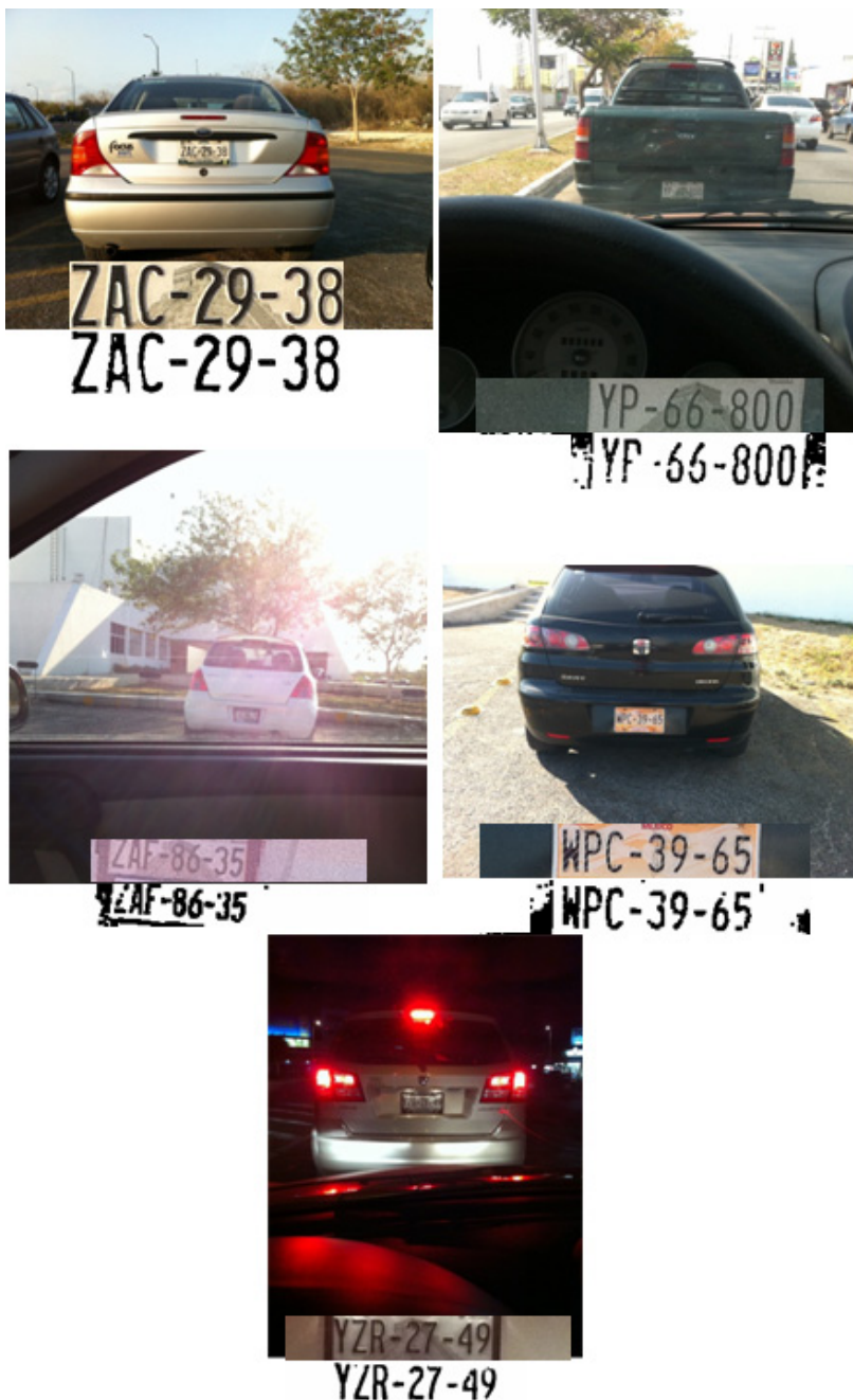
Fig. 3. Image of different cars in different conditions; the identification of the plate region obtained with the proposed method, and results from compact plate region normalization
