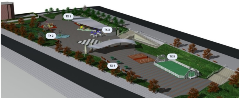
Fig. 3. Scenario under consideration with the representation of the deployment of five readers RFID
