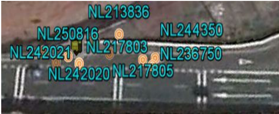
Fig. 3. Point of the route where the vehicle does not have right of way and so it is frequently forced to stop. The orange circles represent vehicle positions at zero speed, the text in green are the labels of these positions (image obtained from GoogleMaps).
