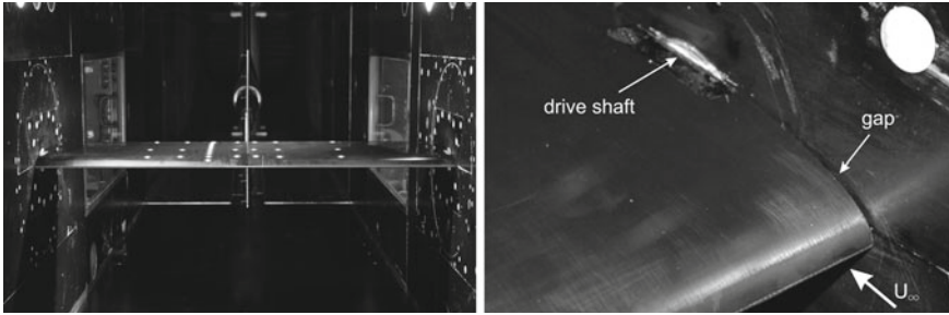
Fig. 1 Rotor blade airfoil model OA209 in the adaptive-wall test section of the DNW-TWG ( left ) and close-up view of the model installation at the wind tunnel side wall ( right )
