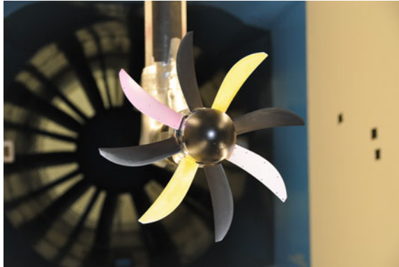
Fig. 8 Picture of the PSP/TSP coated propeller model in the test section of BLSWT
