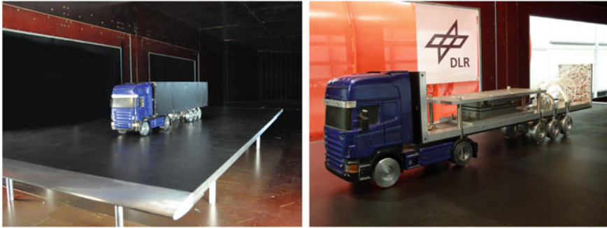
Fig. 1 Wind tunnel setup in the SWG test section
