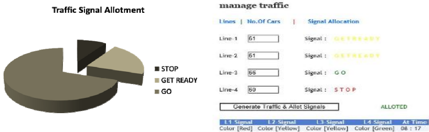
Fig. 5. The results of the priority generated allotting R, G, Y signals in various criteria – More the traffic higher the green signal allotment, optimization of waiting time
