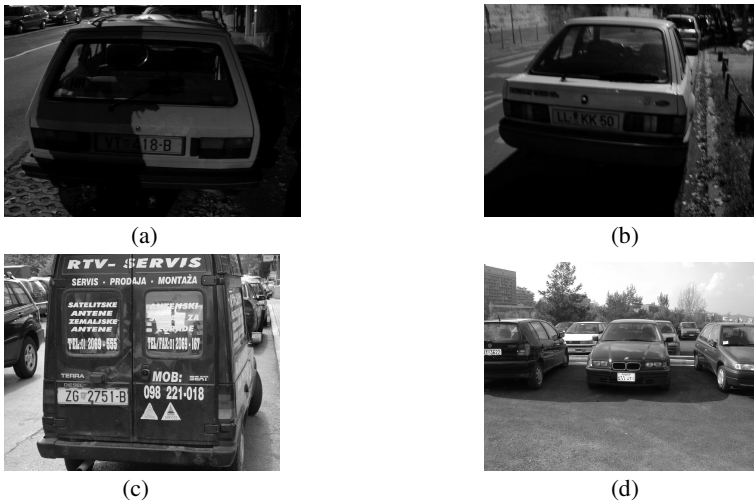
Fig. 5. Examples of failures to localize number plates: (a) number plate partially covered by shadow, (b) poor lighting condition, (c) text around the plate region, and (d) long distance captured image with multiple cars
