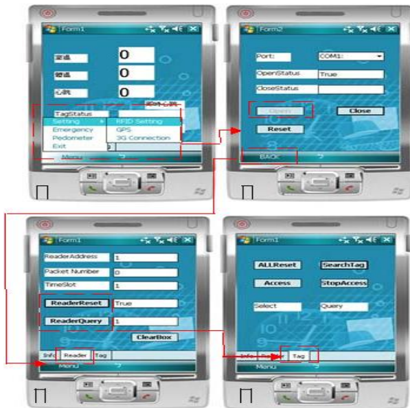
Fig. 5. Setup steps for communication between the smart phone and RFID reader/Tag
