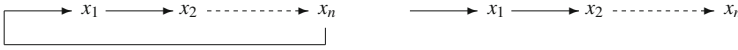
Fig. 2.2 A cyclic system ( left ), built by feedback from a cascade of n systems ( right )
