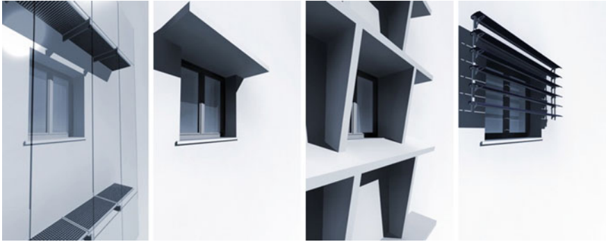
Fig. 11 Examples of fixed shading (from the left horizontal sunshade, fixed overhang, grating and sunshade, fixed blades)
