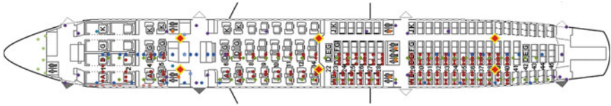
Fig. 2 Setup of access points and wireless sensor nodes in the aircraft
