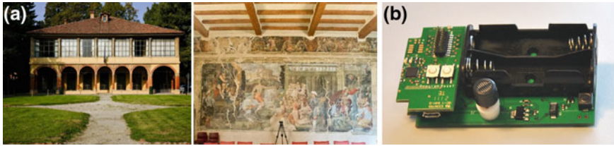
Fig. 1 a Heritage building with WSN deployment. b Hardware unit: A rear view of 32-bit WISPES W24th prototype
