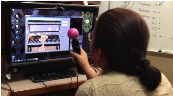
Fig. 1. The Gesture therapy virtual rehabilitation platform for the upper limb. Gesture Therapy characteristic gripper permits controlling of the user avatar through tracking of the colorful ball as well as monitoring gripping forces by an incorporated pressure sensor. Serious games of the platform as the one pictured encourage repetitive exercises beneficial for motor rehabilitation.
