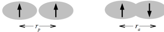
Fig. 1.2 Sketch of two orbitals and the average distance for two different spin orderings
