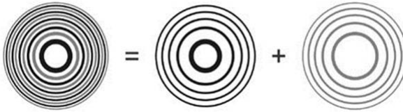
Fig. 5.7 Instead of generating a high density, high aspect ratio FZP in one step, one utilizes the overlay technique, which breaks this process into multiple steps with less demanding properties. However, this can only be met, if a high precision alignment of the ZPs during the multiple steps can be achieved. From [34]
