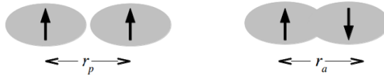
Fig. 1.2 Sketch of two orbitals and the average distance for two different spin orderings
