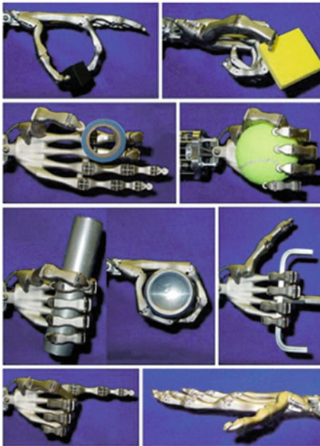
Fig. 4 Six hand grasps and two hand postures, which constitute one of the primary design objectives of the hand prototypes
