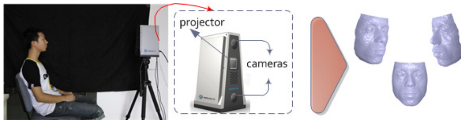
Fig. 3. Capture system and one captured 3D face model with different views
