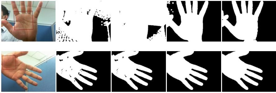
Fig. 8. Dynamical changes of hand binary pictures based on the region learning and the red square is the learning region
