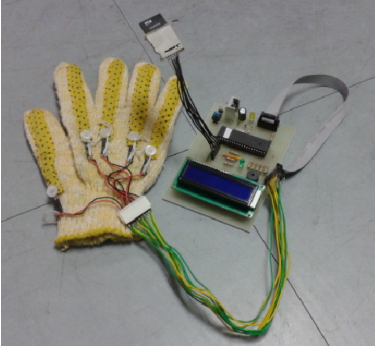
Fig. 7. The completed prototype of the developed standalone sign based recognition system
