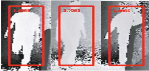
Fig. 5. Examples of persons detection with accuracy of the depth value
