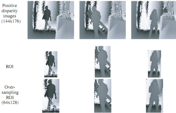
Fig. 3. Positive samples of disparity map with the extracted ROI
