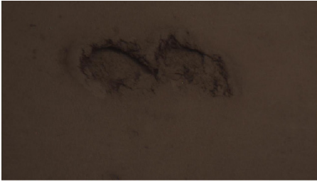
Fig. 5. leather sample at iteration 3 with shutter speed 887.7ms and gain 3.8dB, which is an under exposure with mean luminance 69.9
