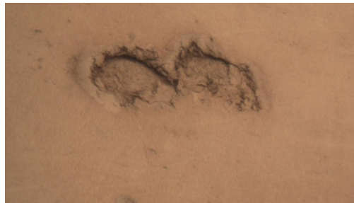
Fig. 7. leather sample at iteration 5 with shutter speed 1355.1ms and gain 6.7dB, which is a proper exposure with mean luminance 132.3
