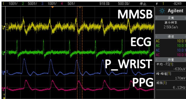
Fig. 1. Snapshot of signals in the oscilloscope (the yellow one is the MMSB signal, the green one is the ECG signal, the blue one is the pressure pulse wave signal and the purple one is the PPG signal).
