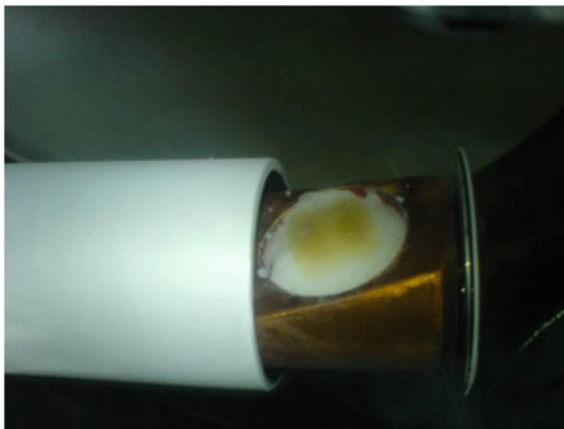
Fig. 11.6 Double-wall target holder used for the growth of the RNase A nanostructures
