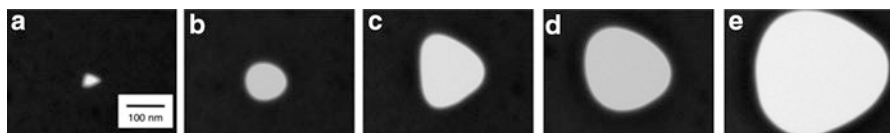
Fig. 15.5 Pattern milling in SiN thin membrane (50nm) by using various spot sizes: (a) 0–0.3 pA, (b) 1 pA, (c) 10 pA, (d) 40 pA, and (e) 80 pA
