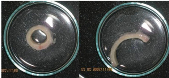
Fig. 4 Arterial ring before carrying out the cut in the radial direction and after releasing of the residual stresses
