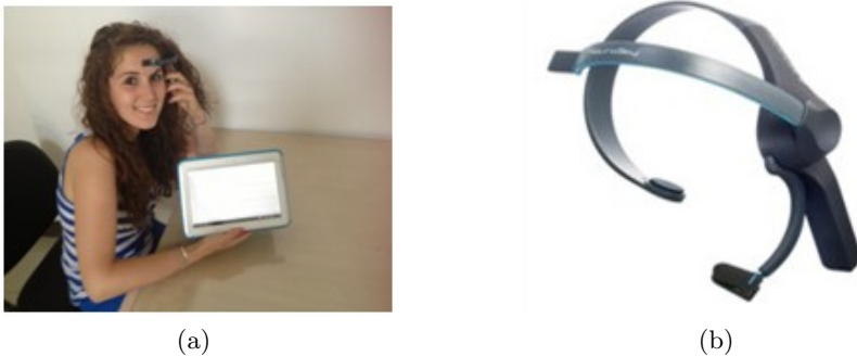
Fig. 1. (a) A participant wearing the MindSet and holding the Sangsun pad based ALMA system. (b) The NeuroSky Mobile MindSet [16].
