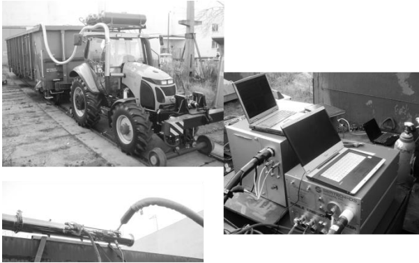
Fig. 6.60 Tests of a Crystal tractor with the emission monitoring equipment installed. The tests were carried out at IPS Tabor in Poznan, Poland.
