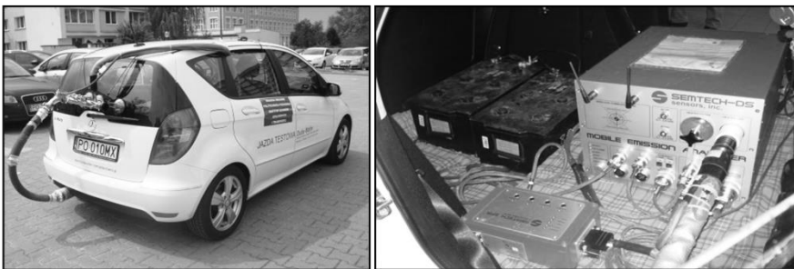
Fig. 6.19 SEMTECH DS fitted in the vehicle for testing
