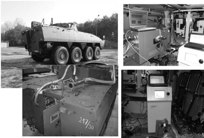
Fig. 6.65 Measurement of exhaust gas pollutant emission from combat vehicles on military training grounds
