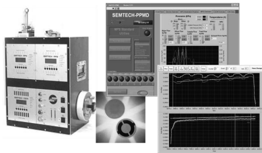
Fig. 6.2 Portable particle measuring device (PPMD) in use (Semtech)
