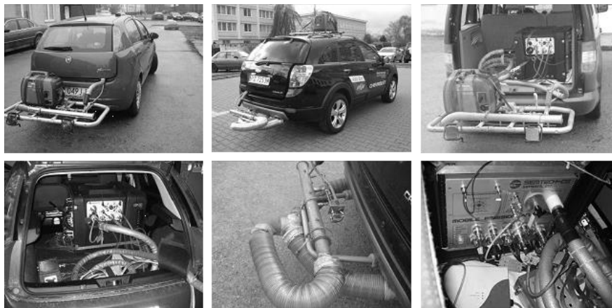
Fig. 6.6 Passenger cars during on-road tests (fitted with various types of internal combustion engines and running on petrol, diesel and CNG)
