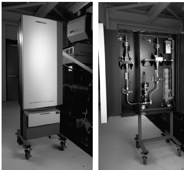
Fig. 4.12 Partial flow system [4]
