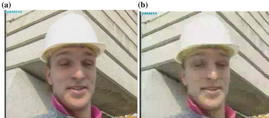
Fig. 19.3 Space varying sensitivity of the HVS to coding artifacts. The blockiness is more visible in flat areas than in high contrast areas as the building wall. a Foreman original frame. b Same frame coarsely quantized
