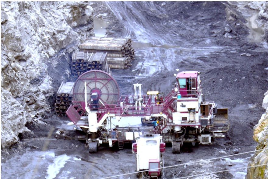
Fig. 1 Highwall face installation showing highwall miner machine at Sharda project
