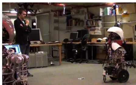
Fig. 1. A training session with the MDS robot Nexi. The artifact used for trainer interaction can be seen on the floor immediately behind Nexi, and the trainer holds a presentation remote by which reward is delivered.
