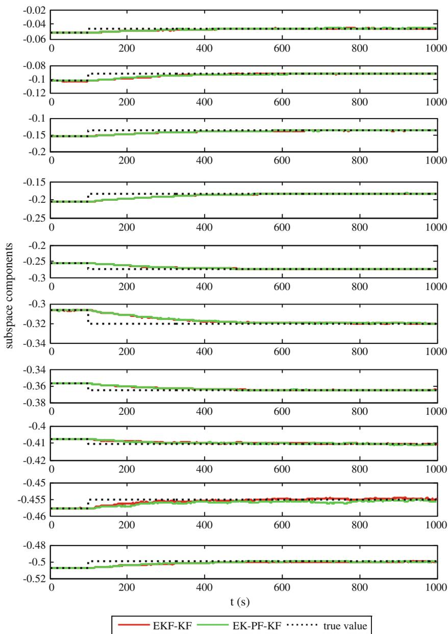
**Fig. 5.7** Time histories of the components of the 1st POM of the structure, from *top* to *bottom* respectively corresponds to first to last component of the POM vector (time histories of entries of POM)
