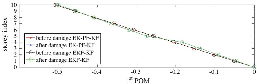
**Fig. 5.6** 1st POM of the structure estimated EK-PF-KF and EKF-KF algorithms
