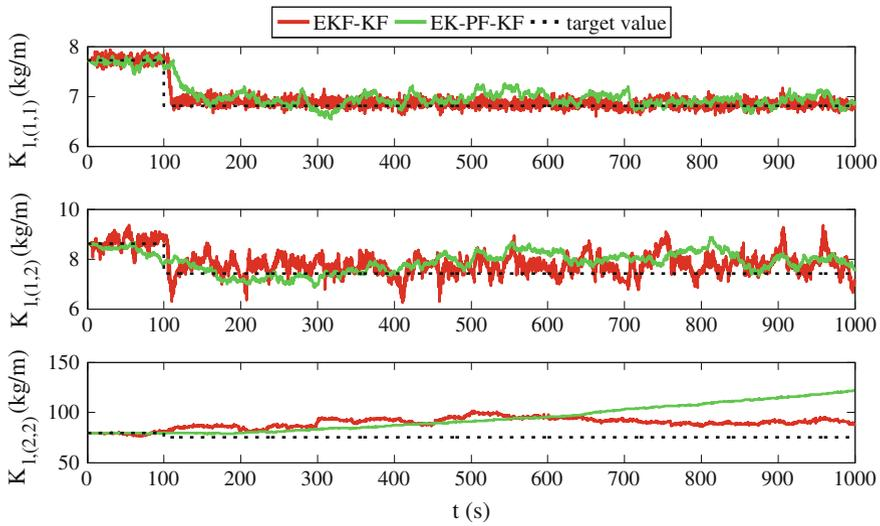
**Fig. 5.8** Time histories of the parameter estimation of the reduced model via EK-PF-KF and EKF-KF algorithms:  $K_{l_i(1,1)}$ ,  $K_{l_i(1,2)}$  and  $K_{l_i(2,2)}$  from top to bottom, respectively
