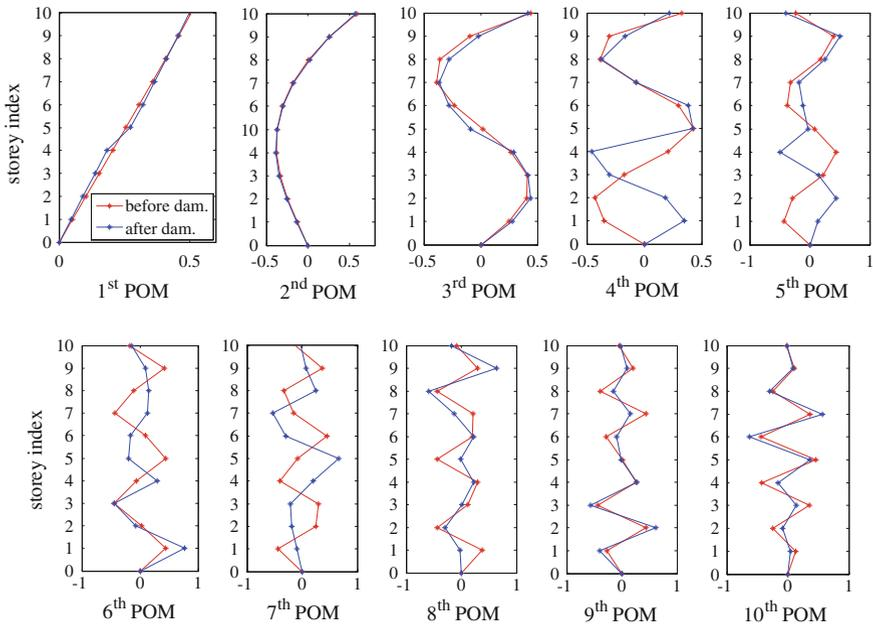
Fig. 5.2 Proper orthogonal modes of a 10 storey shear building before and after damage
