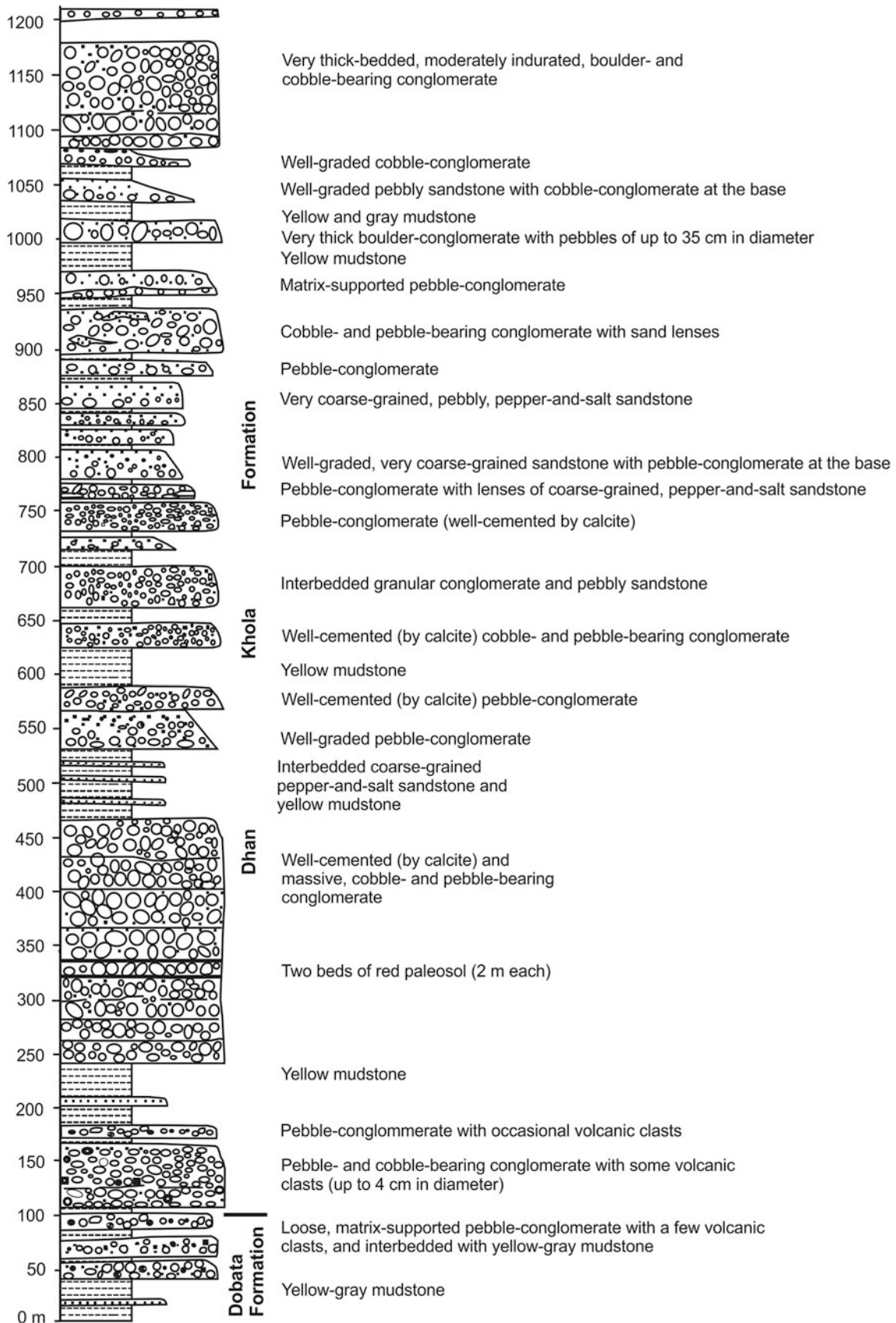
Fig. 29.13 Columnar section of the Dhan Khola Formation prepared from the route maps along the Dhan Khola and the East–West Highway. Notice the considerable amount of mudstone in the middle
