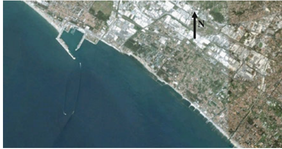
Fig. 8 Port of Carrara, Italy (Source Google Earth). Sediment transport is directed in south-eastern direction. Sand accumulation occurs at the north-western side of the port. The groins on the eastern, downdrift side of the port cover the area with erosion problems
