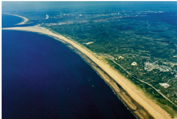
Fig. 7 Port of IJmuiden, sediment transport is directed in northern direction (i.e. towards the top left of the image). Accretion occurs at the south side of the breakwaters (Source RWS)
