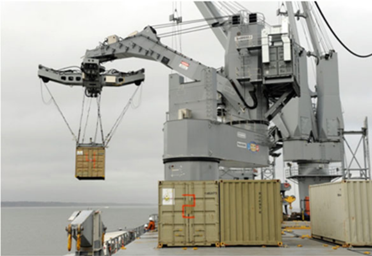
Fig. 5 The large vessel interface lift on/lift off (LVI Lo/Lo) crane for ship-to-ship container transfer at sea ( Source ONR, USA)
