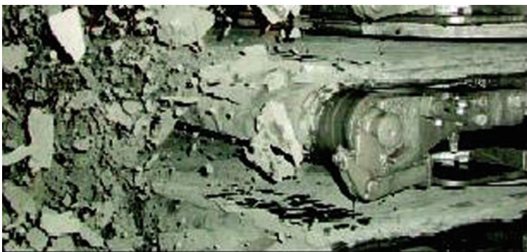
Fig. 9.13 Discharge of the filter cake
