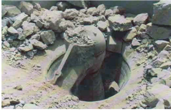
Fig. 1.3 Primary crushing stage: gyratory crusher
