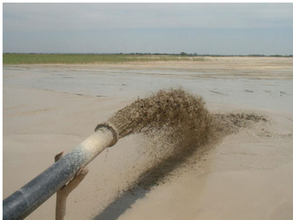
Fig. 1.11 Discharge of tailings into a tailing dam
