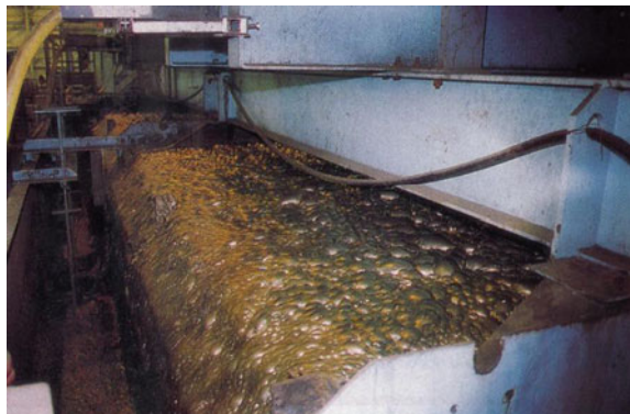
Fig. 1.7 Flotation cell in a copper concentrator
