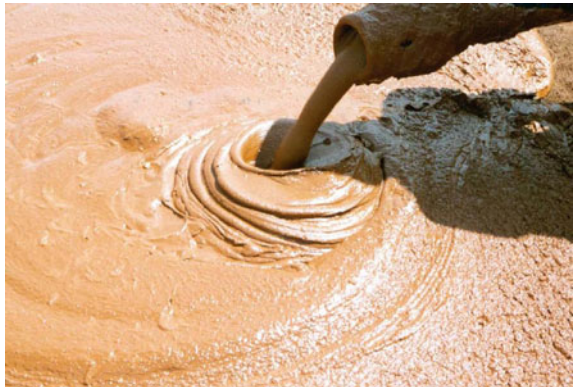
Fig. 1.12 Material behaving as a non-Newtonian tailing
