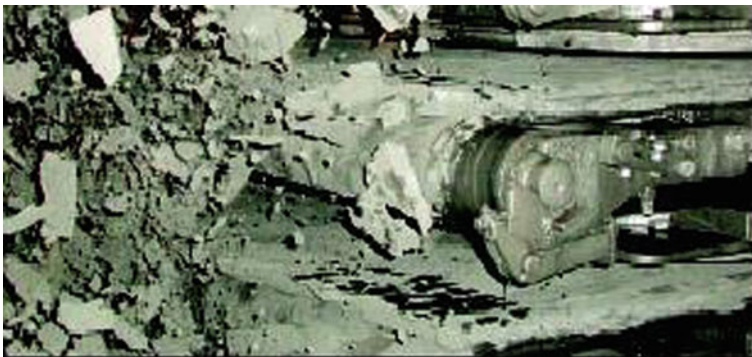
Fig. 9.13 Discharge of the filter cake
