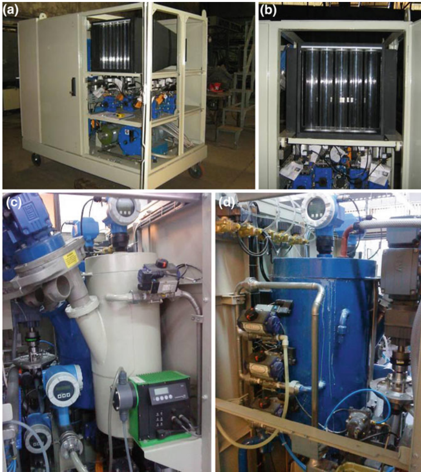
Fig. 8.56 PSE instrument. a General view. b Sedimentation tubes. c Flocculant tank and dose pumps. d Pulp mixing tank
