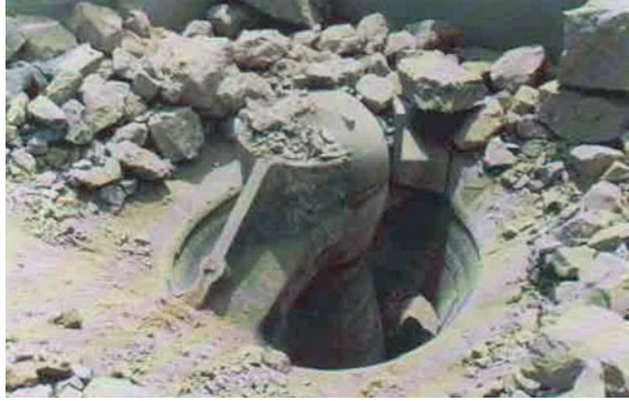
Fig. 1.3 Primary crushing stage: gyratory crusher
