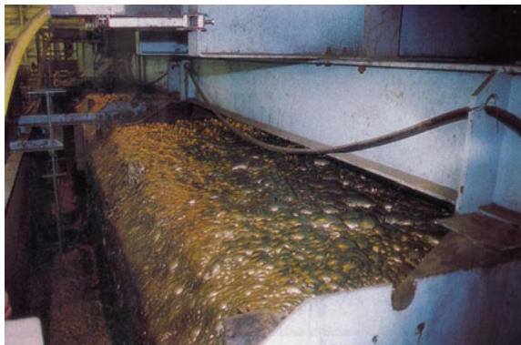
Fig. 1.7 Flotation cell in a copper concentrator
