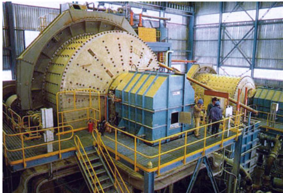
Fig. 1.5 SAG mill in the foreground, with a secondary ball mill at the side
