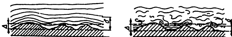
Fig. 11.5 Flow past rough tube walls for different ratios of viscous sublayer to roughness asperity
