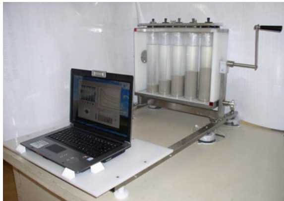
Fig. 8.52 SediRack complete with notebook with webcam
