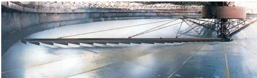
Fig. 8.9 Rakes with lifting system (courtesy of Eimco process equipment)
