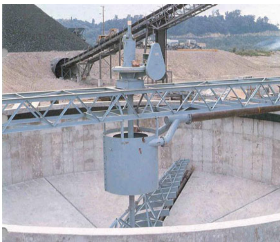
Fig. 8.6 Small thickener with two tangential entries showing centrally driven rakes (courtesy Dorr-Oliver)
