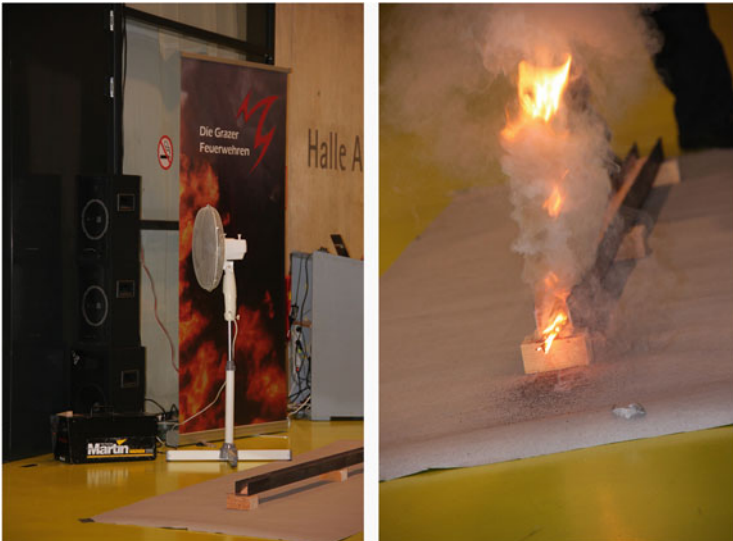
Fig. 2 Installation of smoke generators and speakers in the west foyer (left); ignition of smoke powder (right) (Photos by courtesy of fire brigade of Graz [5])
