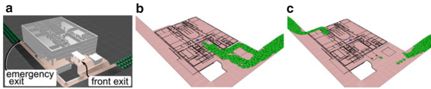
Fig. 5 Phased evacuation from library building. (a) Floor layout. (b) Without guidance. (c) With guidance
