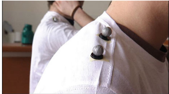
Fig. 2 Each pedestrian is equipped with four markers: two on the right shoulder, one on the right, and one on top of head
