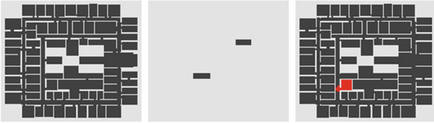
Fig. 2 Illustration of the cellular automaton layers of a two-story building model: the ground floor ( left ) and the first floor ( right ) are connected by a middle layer ( center ) which connects the areas of the staircases in both floors. Empty cells are light gray , unburned cells are dark grey , and burned cells are shown in red
