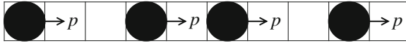
Fig. 6 Schematic view of the TASEP with a parallel-update rule and a periodic boundary condition
