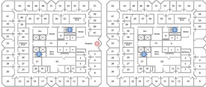
Fig. 1 Illustration of the floor plans of the ground floor ( left ) and the first floor ( right ). The only exit ( E ) of the building is located on the ground floor. Two staircases ( 1 ) and ( 2 ) connect the first floor with the ground floor
