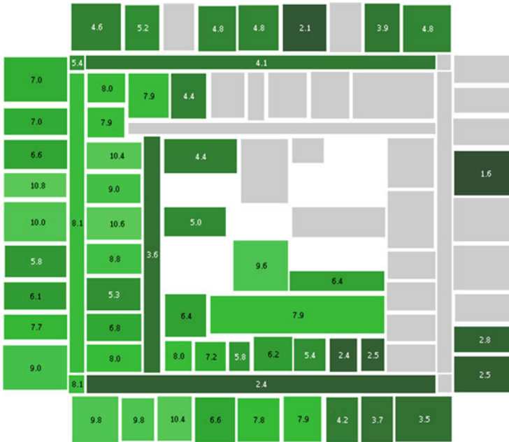
Fig. 5 Heat map indicating the difference in survival rates (if significant) on the first floor, depending on the initial location of the fire. The numbers indicate how much better the guidance system performed (in %). Grey indicates that there has been no significant difference
