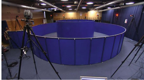
Fig. 1 The experiment room. Two cylindrical walls limit the walking area, surrounded by infra red cameras
