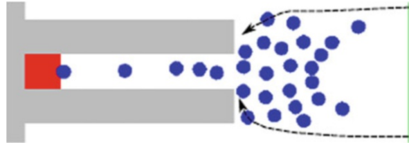
Fig. 4 Two faster pedestrians overtaking on the outside of the congested bneck simulation using the bneckTT parameter set
