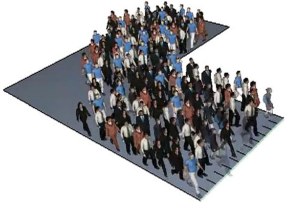
Fig. 2 A Pathfinder simulation where a large group turns a corner, then exits through a series of turnstiles
