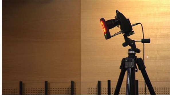
Fig. 3 One of the 12 infra-red cameras of the VICON system that allow to track the markers throughout the experiment
