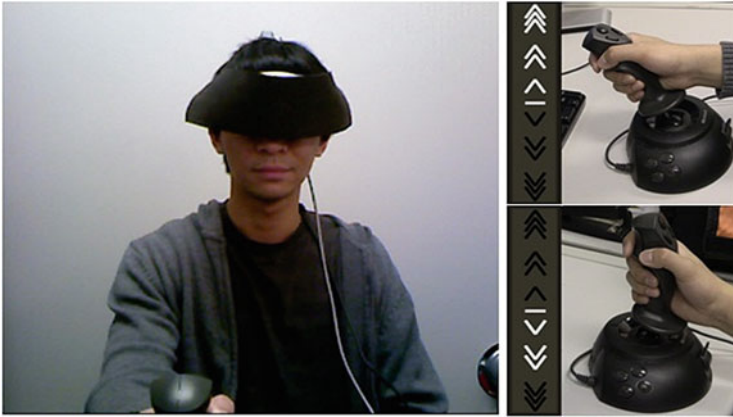
Fig. 2 Participants viewed the virtual library evacuation through a HMD with position tracker attached. When the participant moved the joystick forward, up arrow(s) were displayed, representing a desire to move faster; down positions indicated a desire to slow down. When the participant was moving at a comfortable speed, only the bar in the neutral position was lit
