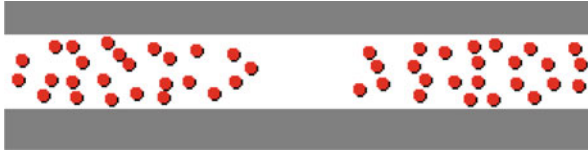
Fig. 1 A 2 m wide corridor with 50 pedestrians was used as a scenario for data creation. Here a simple visualization of the simulation with pedestrians in red and walls in grey
