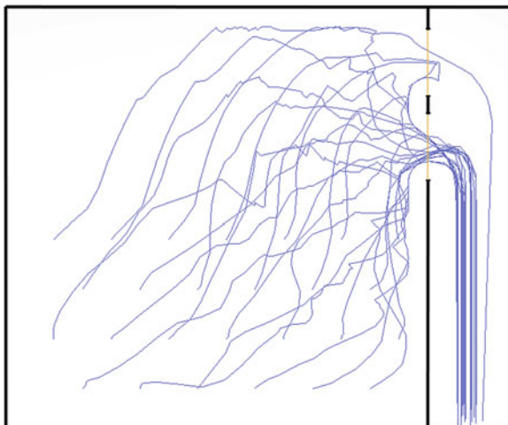
Fig. 1 Shortest-path-only agents fail to utilize the full width of divided doors
