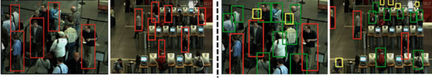
Fig. 2 Left : human detection results using [6]. Right : human detection results using our approach where red boxes show the human detected as full bodies, green boxes show the humans detected as upper bodies, and yellow boxes show the humans detected as heads only. It is clear that [6] failed to detect occluded humans since it does not have an explicit occlusion model, while our approach detects the occluded parts and excludes them from the total detection scores, thus achieving significant improvements especially in crowded scenes
