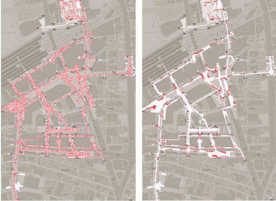
Fig. 8 Crowd flow in large underground shopping mall
