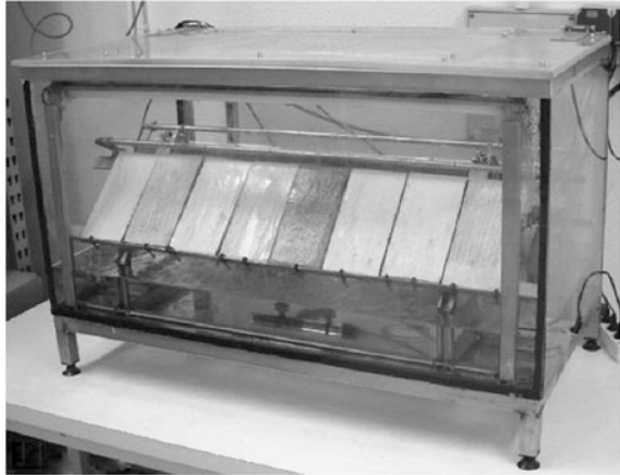
Fig. 5.6 Setup of equipment used by Barberousse et al. to verify the colonisation of the facades by microalgae and cyanobacteria. Reprinted from Barberousse et al. (2007), copyright 2007, with permission from Elsevier
