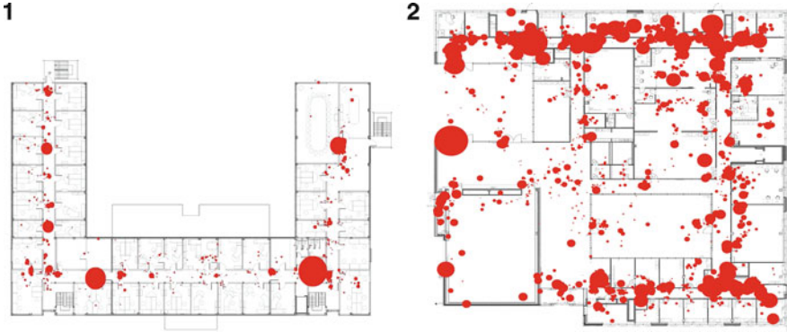
Fig. 7 The floor plans of the models A and B with the locations of vantage points (shown by circles), where participants performed reorientations and explorative turns lasting longer than 1.5 s. The diameter of a circle is proportionate to a number of long turns recorded at its central point
