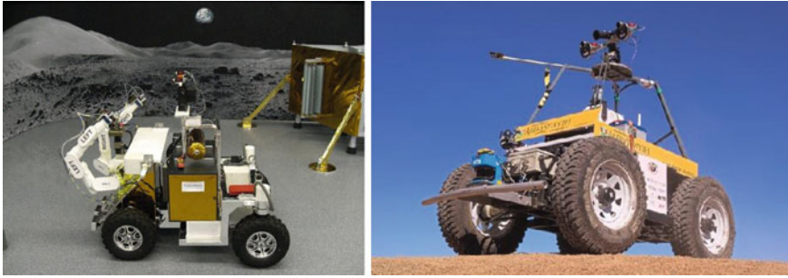
Fig. 4 EGP-Rover over moon-like scenario ( left ) and IDRIS rover at Tenerife final test campaign ( right ) [27]
