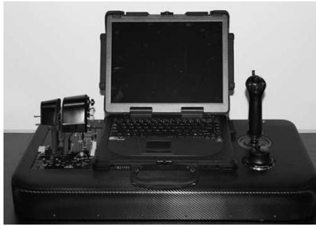
Fig. 3 Complete GCS device with fully-rugged notebook
