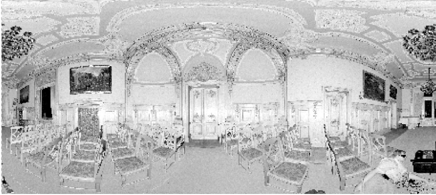
Fig. 2 Scan made by FARO LS scanner – the greylevels represent infrared reflectivity. (Image generated using JRC Reconstructor (R) software.)
