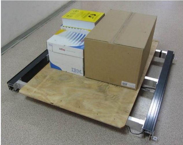
Fig. 9 Mobile Platform under Test Load
