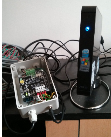
Fig. 4 Host computer; temperature controller and USB/uBus converter based on our own design
