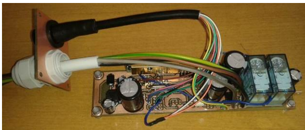
Fig. 8 Control and Power Electronics Board
