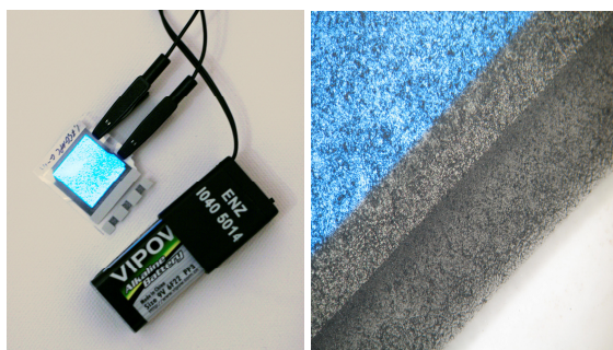
Fig. 7 Electroluminescent displays with screen printed transparent graphene composite electrode
