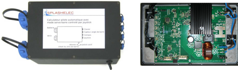
Fig. 2 PSC of the Splashelec system in a waterproof case. It contains several inputs for the keyboard, the compass, the rudder angle sensor, the battery.
